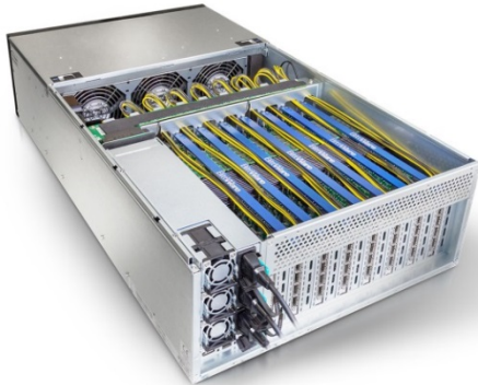
BittWare TeraBox 18M logic elements, 4.9 Tb/sec I/O 8 FPGA cards/16 FPGAs, 2 TB DDR4
